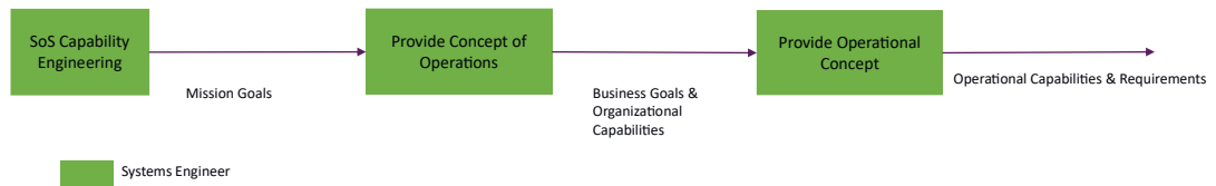
Figure 5: SoS capability engineering to system concept at level 2.
